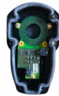
MK2 Encoder (Electric Commercial Vehicles) End application for position correction of Motor Shaft – Designed inhouse
